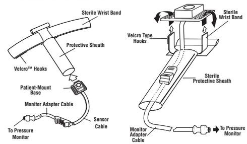
Fig. 3A: Insertion of patient-mount base and monitor adapter cable into sterile protective sheath.
