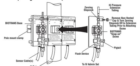
Fig. 4A: Snap Primed Biotrans™ I Dome to Sensor Base
