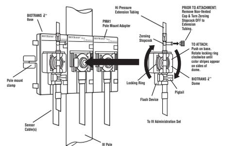
Fig. 4B: Attachment of Primed Biotrans™ II Dome to Biotrans™ II Sensor Base
