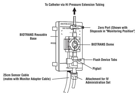
Fig. 1: BIOTRANS™ Pole-mount Base, shown with Disposable Dome in place
