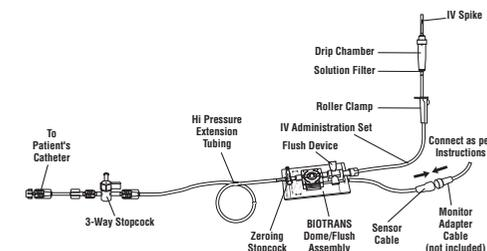
Fig. 2: Typical BIOTRANS™ Disposable Pressure Monitoring Kit, shown without BIOPORT™ Accessory. See Instructions for Assembly and Use.
