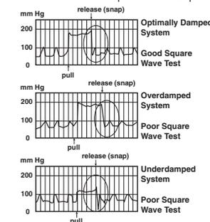
Fig. 5: Waveform response to 'Square Wave Response Test'. See text for details.
